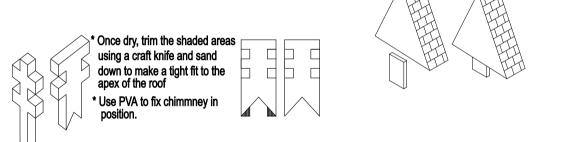
Glue in small 3mm blocks to inside of gables leaving 5-10mm protruding
