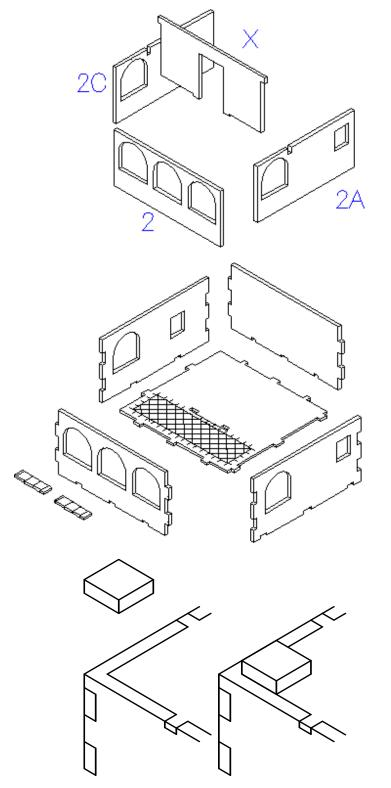
TIP: Do not glue in the inner dividing wall marked with an X on the diagram.
