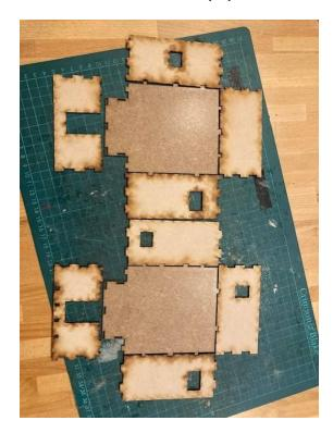
All kits with pent (single slope roof) have the convention of lining pieces being identified as follows: G = ground floor, working counter clockwise, GA, GB and GC. Ist floor and  $2^{\text{nd}}$  floor have had 1 or 2 engraved on the pieces rather than G.
