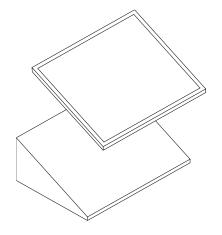
Glue the rectangular 3mm piece to the underside of the roof using a general-purpose adhesive or epoxy resin.
