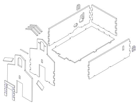
Glue the 3 jointed 3mm external walls to the 2mm base. Next, glue in the 2mm front with the horizontal slot through the bell opening.
