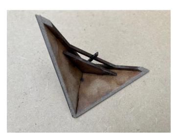
File or emery board the two triangles leading top edges (like the roof) then assemble It is recommended that the front A frame trim is glued in at this time. This makes the sub-assembly 4 pieces in total.
