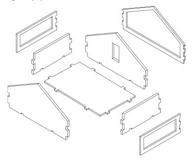
Glue together to two first floor small rooms and set aside to dry.
