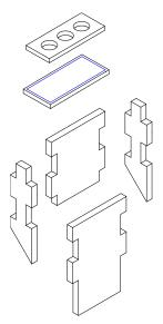
Glue the 4 3mm pieces and cap with the blanking rectangle. On top of this glue on the top piece and glue in the plastic chimney pots. (Use a general purpose glue or superglue for this step.)
