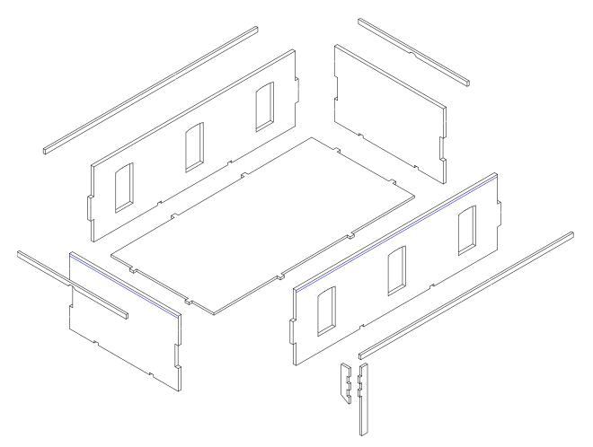
Assemble the middle upper floor and glue on the long strip trim under the engraved line (shown blue). The corner "blocks" will interlock and should be aligned to the underside of the long strip. The longest pieces of vertical trim should also align with the base of the wall. NOTE: the side trim has a "n" curve in the middle. Ensure this is the right way up and NOT INVERTED as a "u".
