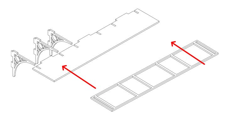
NOTE: when "posting" the top trim to cover the acrylic, apply SLIGHT pressure if needed by pressing where there is a strut. Do not apply pressure in between struts.
