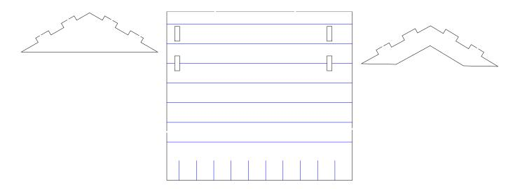
Glue the two triangular sides to the clock housing to the front roof. Glue on the front piece with the engraving facing the outside.
