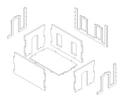
Set the lower 3 room sub assembly aside to dry and now work on the top 3 rooms.
