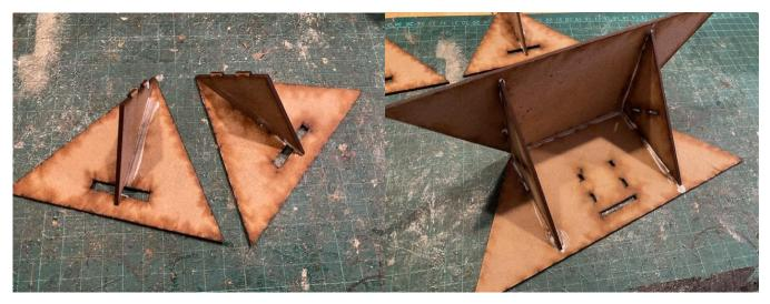
Glue on the two sloping side roof sub-assemblies and run a bead of PVA along each seam.
