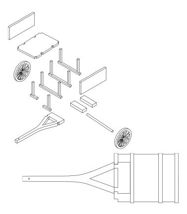
Glue in the 3mm rectangles between the support struts, giving a 2mm channel to accept the axle.
