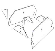
For the roof assembly, glue in the hipped roof supports to either end. Glue both ends and the
