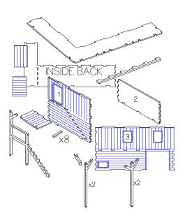
Glue the steps side part 1 to the inside back, ensuring that the planks are on the outside. Glue on part 3 followed by part 2. With the floor, planked side face up, and planks nearest you; glue in the ground floor assembly.
