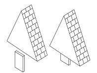
Glue block to inside of gable opposite the chimney wall leaving 5–10 mm protruding.
