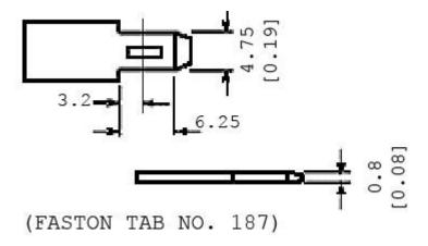
**The F1 Faston Tab is No. 187** because it is 0.187" wide. This is equivalent to 3/16" or 4.75 mm. If your application requires the larger, F2 terminal type, there are adapters available to attach to the F1 and make it compatible with F2 connectors.
