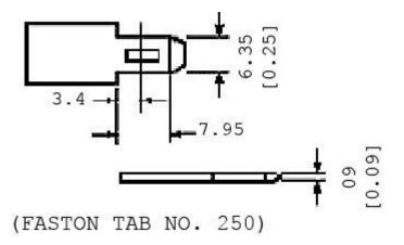
**The F2 Faston Tab is No. 250** because it is 0.25" wide. That's 1/4" or 6.35 mm. The difference between the F1 and the F2 is only 1/16". That difference in width may appear to be miniscule, but if the application calls for one or the other, we recommend sticking to it.
