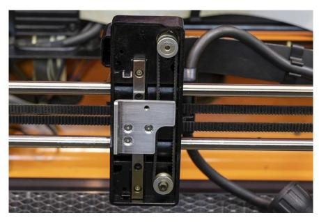
Belt installed over motor and lower pulley.
