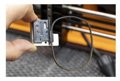
Install belt onto new bracket.
