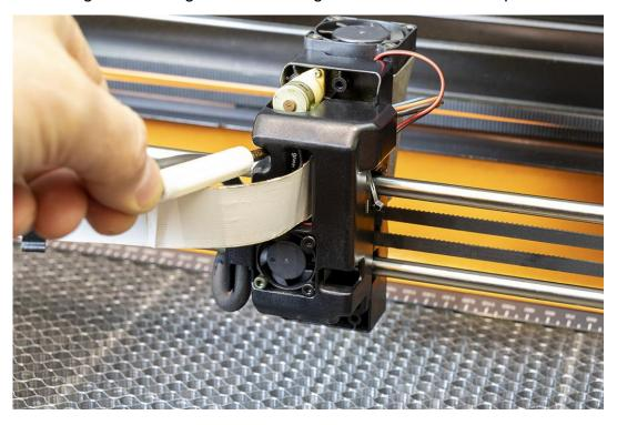
Removing the upper left screw holding the rear laser cover in place.
