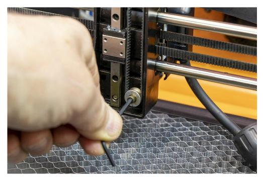
Unscrew the lower belt pulley.
