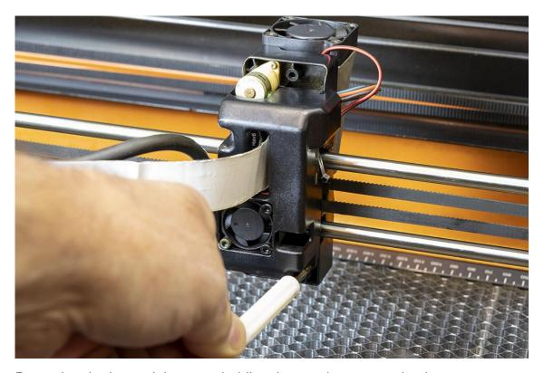
Removing the lower right screw holding the rear laser cover in place.
