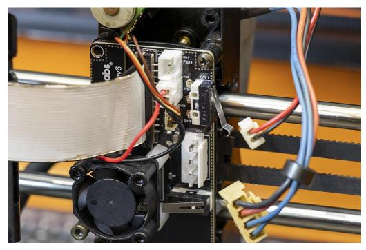
Laser Unit & Fan connectors unplugged.
