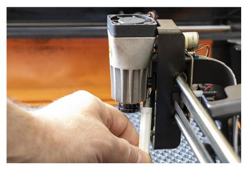
Unscrew bold holding 5w laser unit in place.
