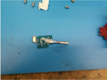
6. Insert the new heating element into the heater block and put the screws in. Don't be afraid to bend the wires a little so the wiring fits in properly within the small square cutout on the heating block. It should like the picture below once done. Also, make sure that the heating element doesn't extend out the other side of the block.
