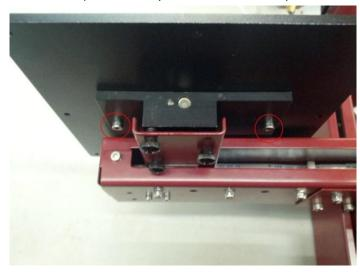
2. Next, you will want to remove the arm cover. Remove the 3 screws circled on the picture below; leave the one in the upper left side alone. After that remove the cover gently to prevent scratches.
