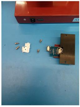
5. Take new Platform Heater you have (Should look like the one pictured below) and bend the heater and thermoresistor forward. Once that is done it should look like the second picture below.
