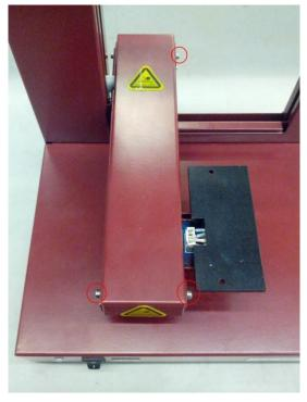
3. Once that's removed you will see the inside of the arm, move the platform heater all the way to the front of the machine. Then you will want to remove the 4 screws circled in the first picture below, the ones attached to the movable platform heater board. Careful as once these 4 screws are removed the heater block will be free and might fall down. Keep track of where the screws go as the two to the Left are longer than the two on the Right. It should look like the 2nd picture once removed.
