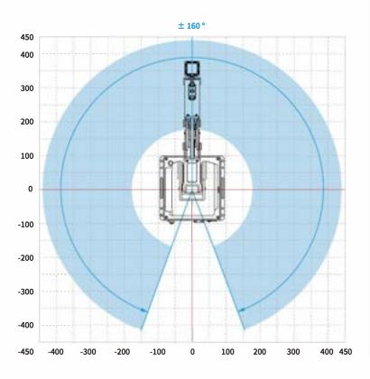
Product Name DOBOT MG400 Product Model DT-MG400-4R075-01 **Controled Axes** Rated Load 500 g (Max. 750 g) Max. Reach 440 mm Repeatibility  $\pm 0.05\,\mathrm{mm}$ **Motion Parameters** Joint Motion Range Max. Speed J1 300 °/s  $\pm 160^{\circ}$ J2 -25°~85° 300 °/s -25°~105° J3 300 °/s -360°~360° 300 °/s
