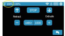
6\ Gently push the filament into the filament entrance and down until it stops. After reaching the print temperature, the printer will beep and start extruding filament.
