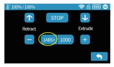
5\ After selecting the right material, click "Extrude". The print head temperature will be displayed on the status bar on top.
