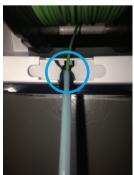
3\ Insert filament and guiding tube into the machine through the hole on the back door.
