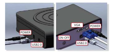
Plug the power cable, VGA cable, and USB cable into the specified connections on the scanner and turntable. Plug the other ends of the cables into the computer and outlet. Turn on the scanner by pressing the power button twice.
