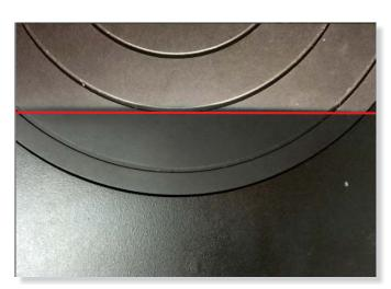
Adjust the angle of the scanner so the lower edge of the projection approaches the second loop of the turntable; tighten the scanner mount bolt.
