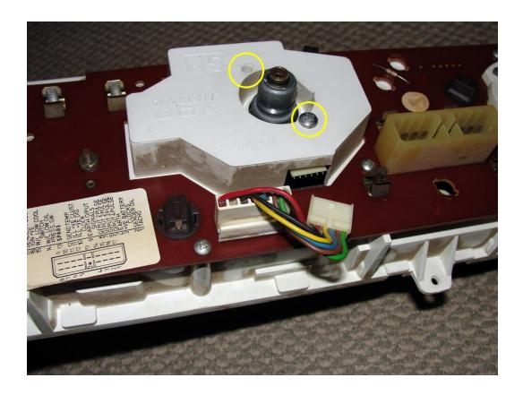
9. Gently remove speedometer with its fascia in one piece. Lift by the edges of the fascia. With the cluster face facing up, pull assembly up gently until the speed sensor gets caught, then turn slightly anti clockwise and wriggle it out by pulling slightly to the right.
