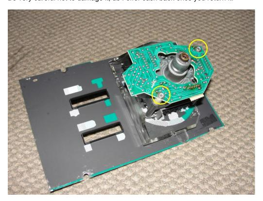
11. Fit new speed sensor, and follow instructions in reverse order to reassemble instrument cluster.
