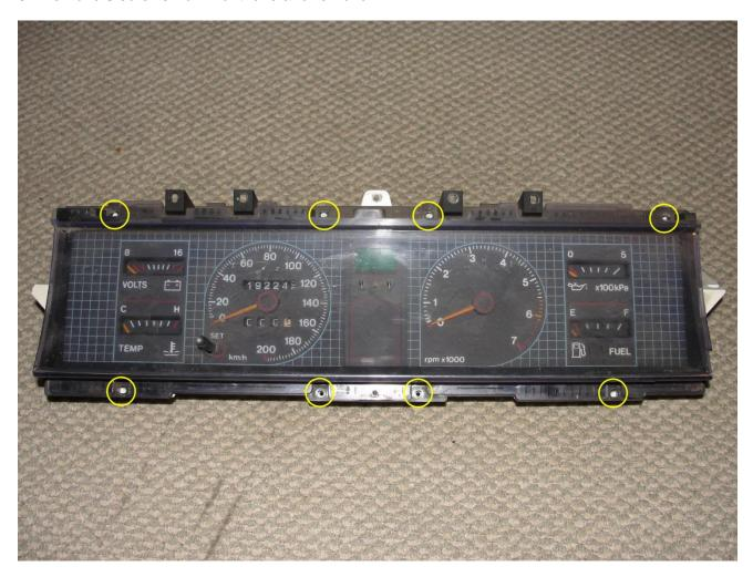
4. Slide the two fascia separators up to remove.
