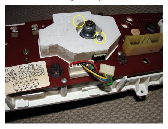
9. Gently remove speedometer with its fascia in one piece. Lift by the edges of the fascia. With the cluster face facing up, pull assembly up gently until the speed sensor gets caught, then turn slightly anti clockwise and wriggle it out by pulling slightly to the right.
