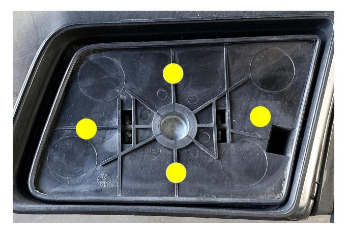
4. To fit the new glass - insert the sharp corner first (1), then snap corner (2) next. Final step is to push corners (3) and (4) down. <u>Be VERY CAREFUL,</u> the glass will break if too much pressure is applied.
