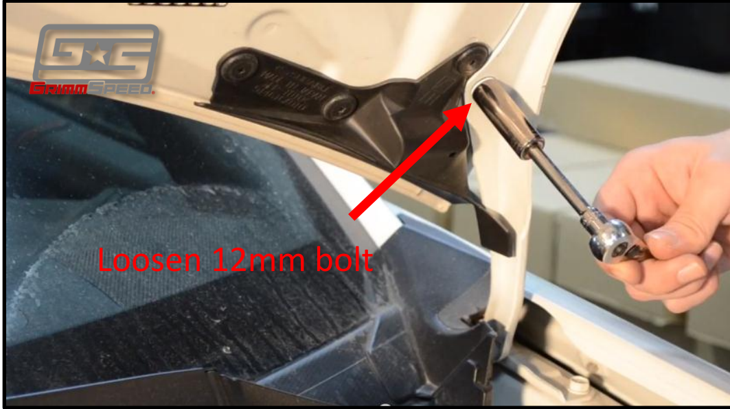
Figure 10: Loosen lower hood hinge bolt.
