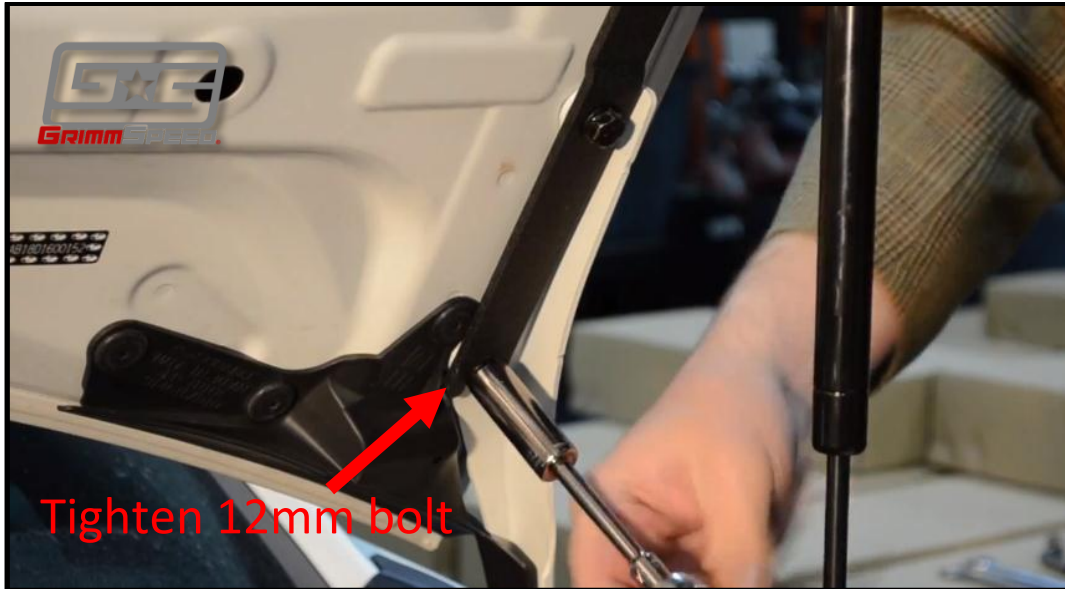
Figure 13: Loosen lower hood hinge bolt.
