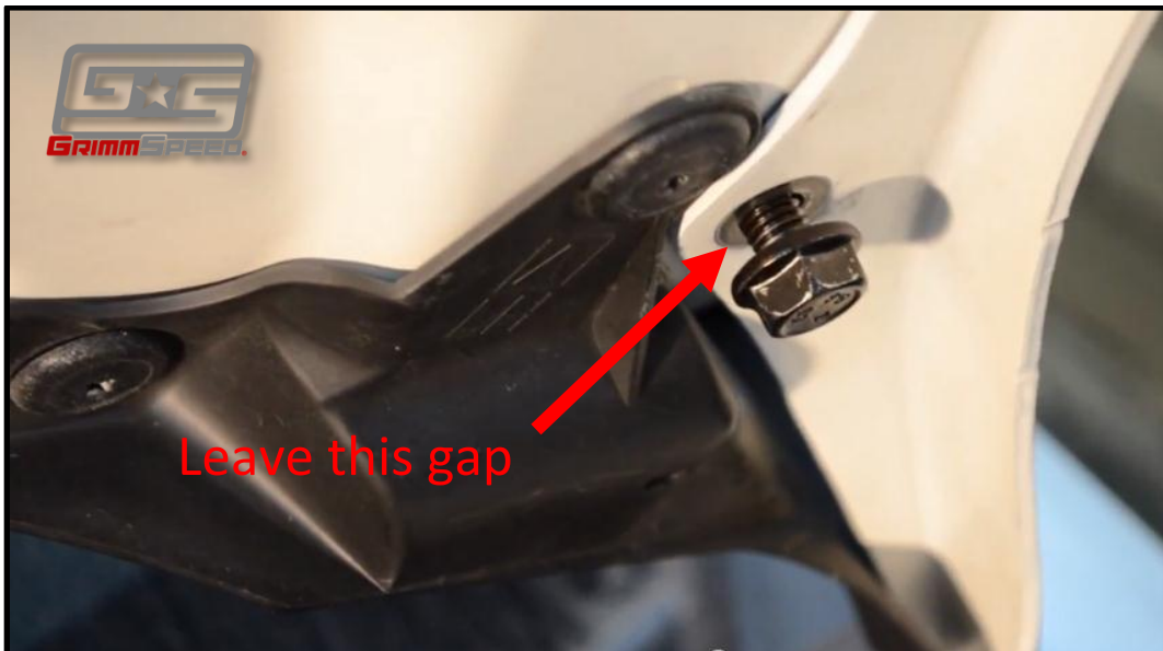
Figure 11: Install lower hood hinge bolt.
