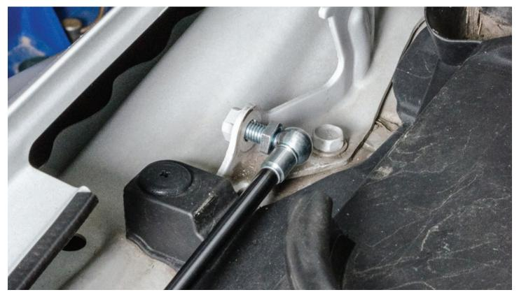
**STEP 6** - Once you have the lower [skinny] end of the strut threaded in most of the way by hand, you can tighten it the rest of the way using a 13mm wrench.
