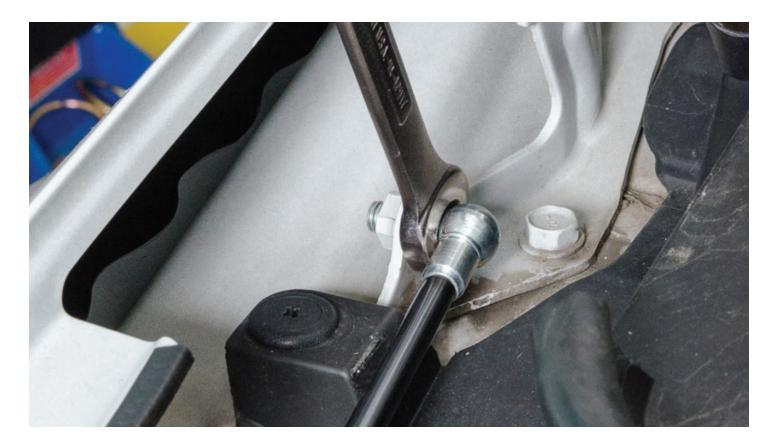
**STEP 7 -** Bolt the top of the strut to the new hood bracket using one of the included nuts. Tighten the upper ball joint down by holding the stud in place with a 13mm wrench and tightening the nut with either another 13mm wrench or socket. Ensure that the ball on the strut in on the outside of the bracket as shown.
