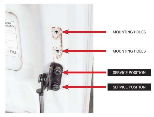
**STEP 3 -** Back on the passenger's side, unscrew and remove the bottom bolt from the chassis using your 12mm wrench. Remove the OEM strut from the car.
