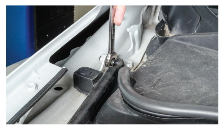
**STEP 4 -** Prep the new GrimmSpeed hood bracket by installing the factory paper washers onto two of the bolts included in your kit as shown below. You can now install this bracket onto your hood in the upper pair of mounting holes, ensuring that the bent tab on the bracket faces the center of the vehicle.
