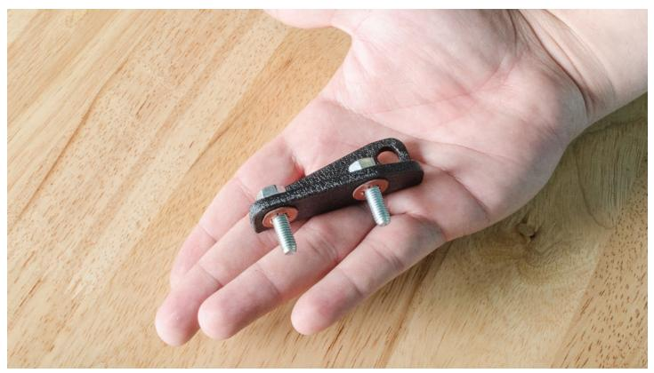
**STEP 5** - Begin installing one of the GrimmSpeed Struts into the factory lower strut bracket. **Ensure that** you are threading in the SKINNY end of the strut on the bottom as the threads are different and you will damage these threads if you have the strut backwards.
