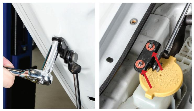
**STEP 2 -** Move to the drivers side and loosen the 2 top bolts on the hood. Notice that there are 2 different sets of screw holes on each side; the top set are the mounting holes, while the bottom set are the service position holes. Move the factory strut on the driver's side to the service position. This will help hold the hood up while working on the passenger side strut.
