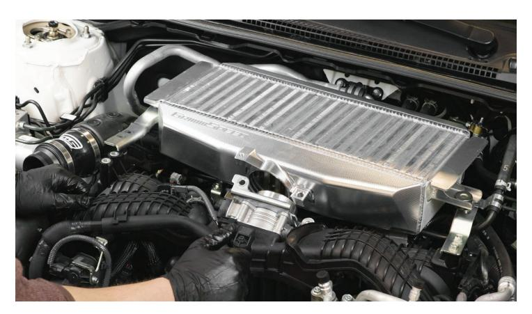
**STEP 17 -** With the intercooler in place, slide the throttle body flange down over the throttle body. This should be a snug fit, so you will need to use a fair amount of force to get it fully seated so the bolt holes line up. **NOTE: If it's too tight or binding up, you may need to apply extra lubrication to the o-rings inside of the intercooler flange.**
