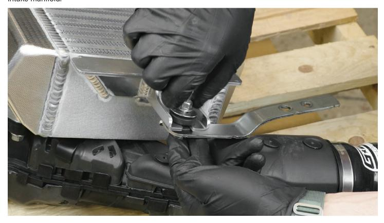
**STEP 16 -** Back under the hood, place the intercooler roughly in place on top of the engine. Ensure that the passenger side support bracket is roughly in place above the intake manifold.
