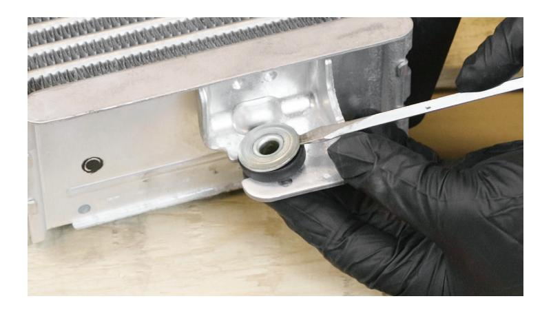
**STEP 7 -** Remove the rubber bushing from the factory intercooler by sliding it out of the cutout slot in the bracket. Repeat step 6-7 on the other side of the intercooler as well so both bushings and sleeve pairs are free.
