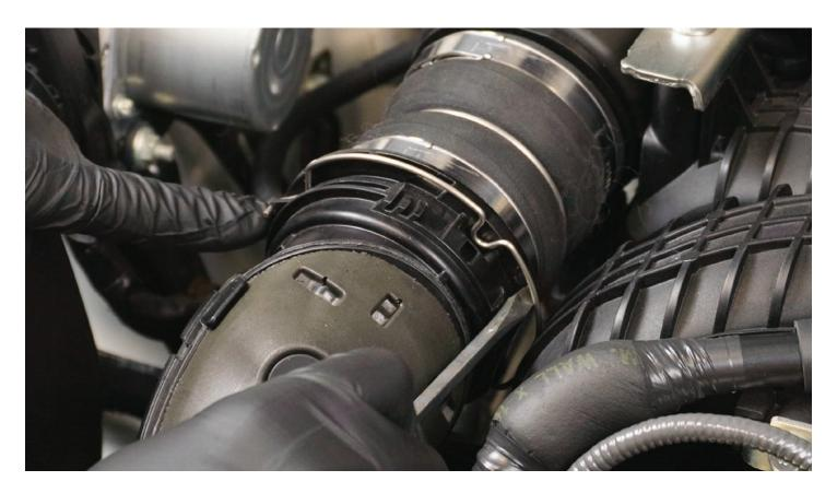
**STEP 2 -** With a 12mm socket, remove the 5 bolts indicated below (2 holding the passenger side support bracket to the intake manifold, 2 on the throttle body, and one mounting the intercooler to the driver's side support bracket)
