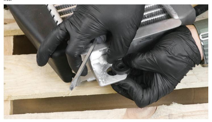
**STEP 8 -** Using your flat head screwdriver or an 7mm socket, remove the clamps from the rubber coupler on the chargepipe.
