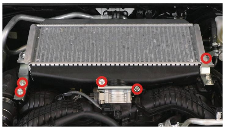
**STEP 3 -** With those bolts removed and the chargepipe disconnected, you should be able to pop the intercooler off of the throttle body (towards the firewall) and remove it from the engine bay.
