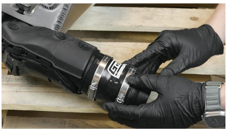
**STEP 15 -** Loosely install the passenger side bracket onto the GrimmSpeed TMIC using another one of the 12mm bolts from before. Finger tight is fine for now as the bracket will need to be loose to mount onto the intake manifold.
