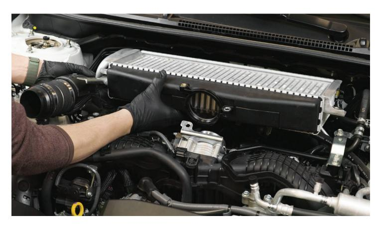
**STEP 4 -** With the intercooler off the car, turn it over and remove the 3 12mm bolts securing the chargepipe to the upper endtank.
