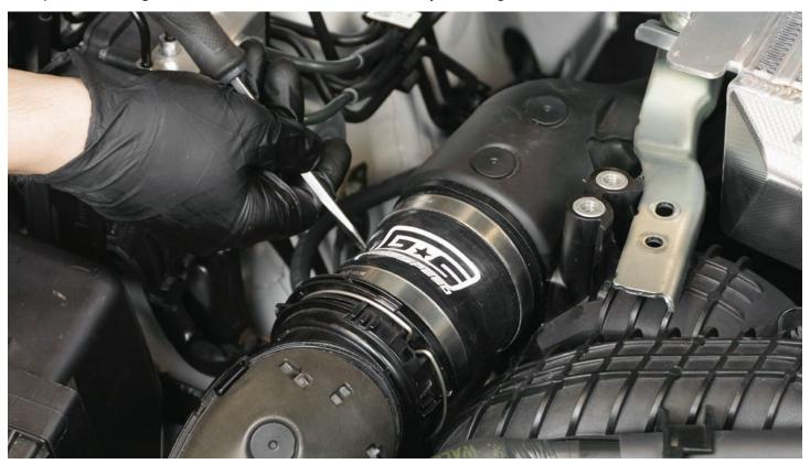
**STEP 20 -** Go through and reinstall the 5 remaining 12mm bolts to secure the GrimmSpeed Intercooler into the car. Don't forget to fully tighten the bolt we installed loosely on to mount the passenger side bushing to the intake manifold bracket. Torque all of the bolts to 11.8 ft/lbs (16 nm)
