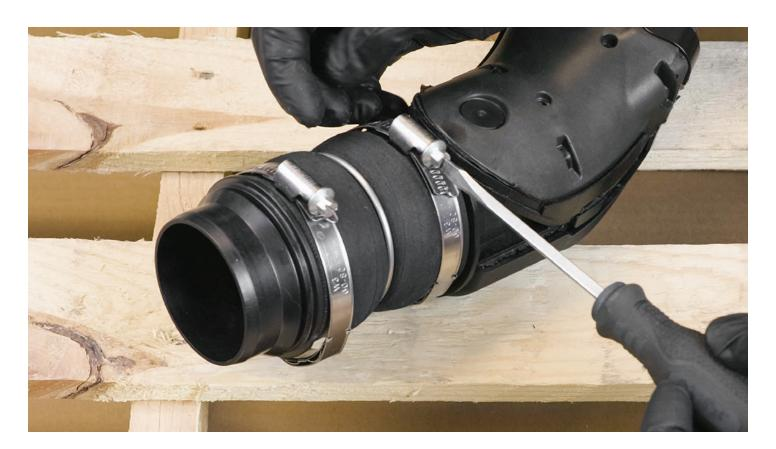
**STEP 9 -** With the clamps loose, separate the chargepipe from the rubber coupler. Remove the quick release adapter from the factory coupler as well.
