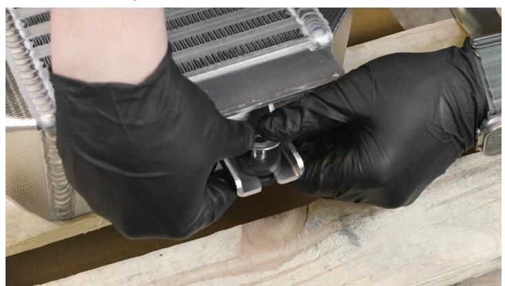
**STEP 11 -** Ensure that the factory o-ring gasket on the chargepipe is still in place and free of any debris before bolting the chargepipe up to your GrimmSpeed Intercooler.
