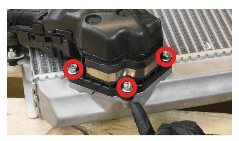
**STEP 5 -** Remove the 12mm bolt securing the support bracket to the end of the factory intercooler.
