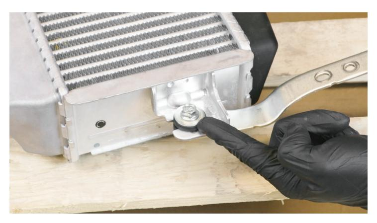
**STEP 6 -** Use a flat head screwdriver to gently pry the metal sleeve out of the intercooler support bushing.
