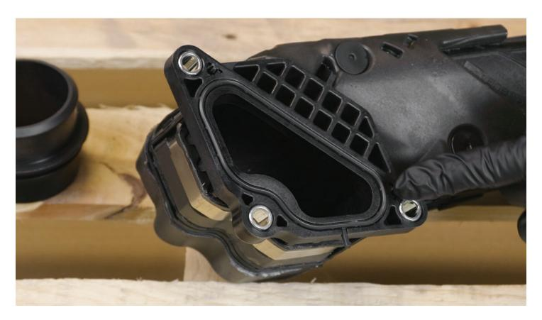
**STEP 12 -** Using 3 of the 12mm bolts you removed eariler, bolt the chargepipe onto the GrimmSpeed Intercooler, ensureing that the two dowel posts on the chargepipe are aligned with the pockets on the intercooler. Torque these bolts to 11.8 ft/lbs (16 Nm).
