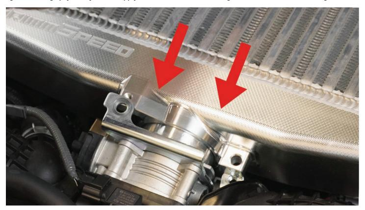
**STEP 18 -** Pop the chargepipe coupler back into place in the lower half of the charge pipe. Once it is seated, you can click the retaining ring back into operating position to secure the adapter. You should hear an audible click from each end of the clip as it enganges.
