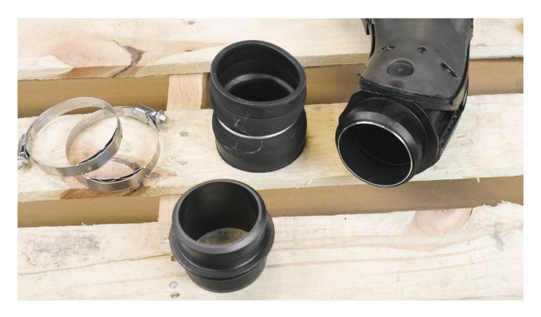
**STEP 10 -** Take the bushings and sleeves you removed in steps 6-7 and install them onto both ends of your GrimmSpeed intercooler. Ensure that the flat sides of the sleeves are facing the front (the side of the intercooler with the GrimmSpeed text).
