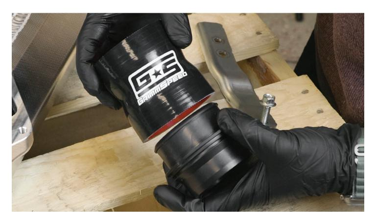
**STEP 14** - Pop the other side of the coupler onto the top side of the charge pipe with the GrimmSpeed logo facing up. Slide the included clamps over the coupler, but don't tighten them quite yet in case you need to re-orient the coupler once the intercooler is on the car.
