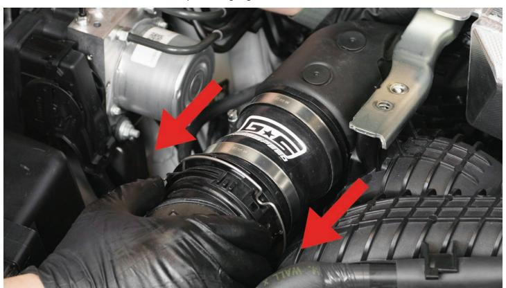
**STEP 19 -** Take a moment to double check that the GrimmSpeed silicone coupler is oriented properly with the logo facing up and then align the clamps so 1/8-1/4" of the coupler is showing on the outside. Tighten the clamps down using a screwdriver or 7mm socket until they are snug. **DO NOT OVER TIGHTEN!**
