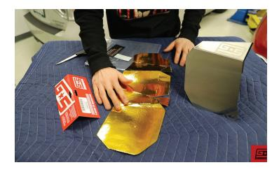
2. Use a pair of scissors along the perforations to cut the foil into pieces.
