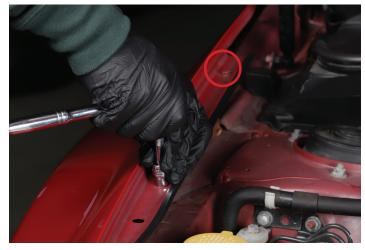
2. Slide the GrimmSpeed Fender Shroud between the fender and the support bracket underneath. Align the holes and reinstall the two 10mm bolts.
