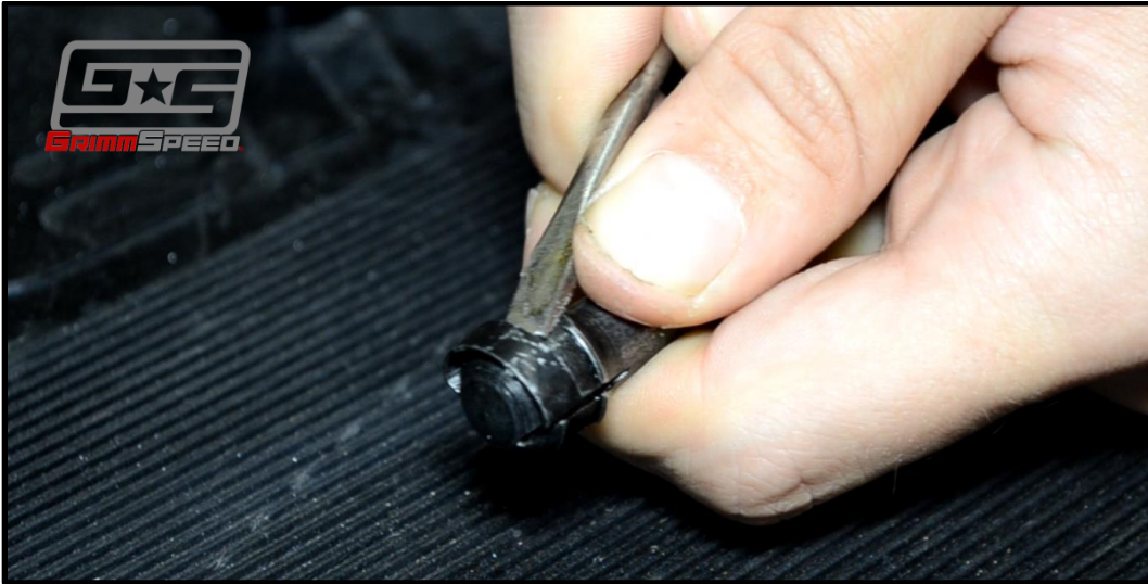
Figure 2: Release socket clips
