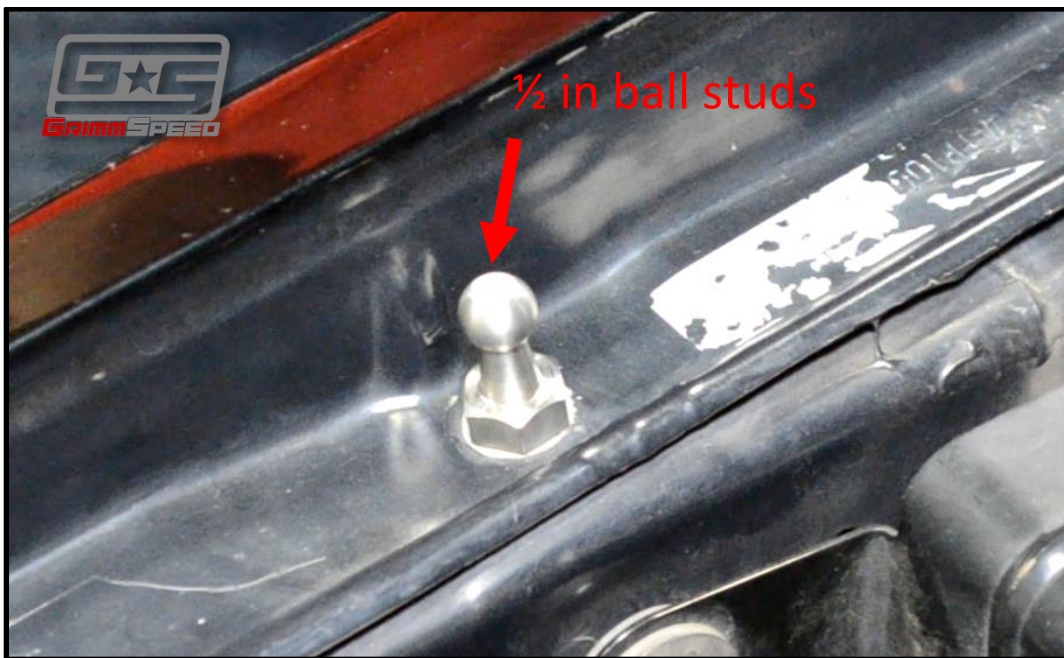
Figure 5: Install ball studs
