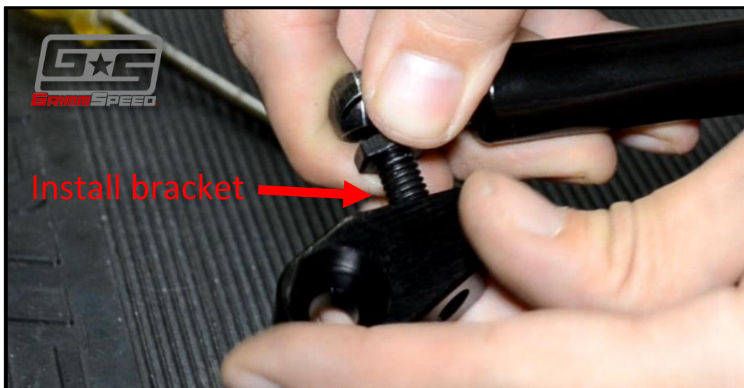
Figure 3: Installing rubber bumper
