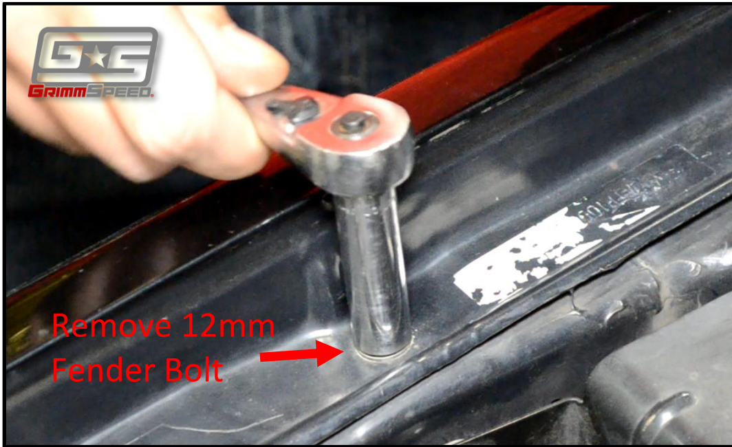
Figure 4: Remove fender bolts
