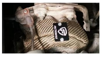
Optional. Stock Heat-Shield can be mounted over the blanket covered turbo.
