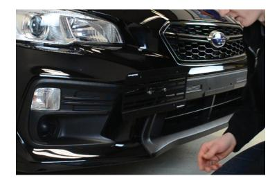
6. With the last 4 included allen screws, attach your license plate and frame to your relocation kit
