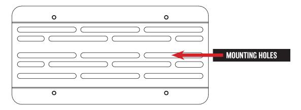
Using the 2 included short 5mm allen bolts, attach the plate to the U-bracket.
