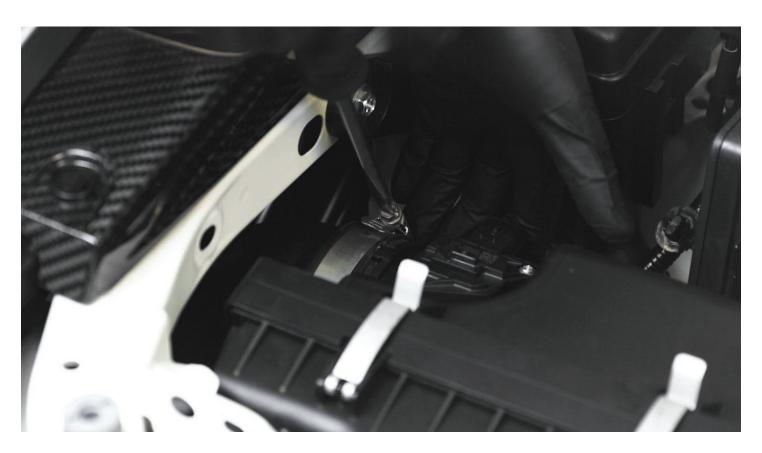
**STEP 10 -** Remove the 10mm nut from the mounting grommet securing the airbox to the bracket behind the headlight. With this removed, you can pop the factory post-MAF pipe off the the airbox and wiggle the box out of the engine bay.
