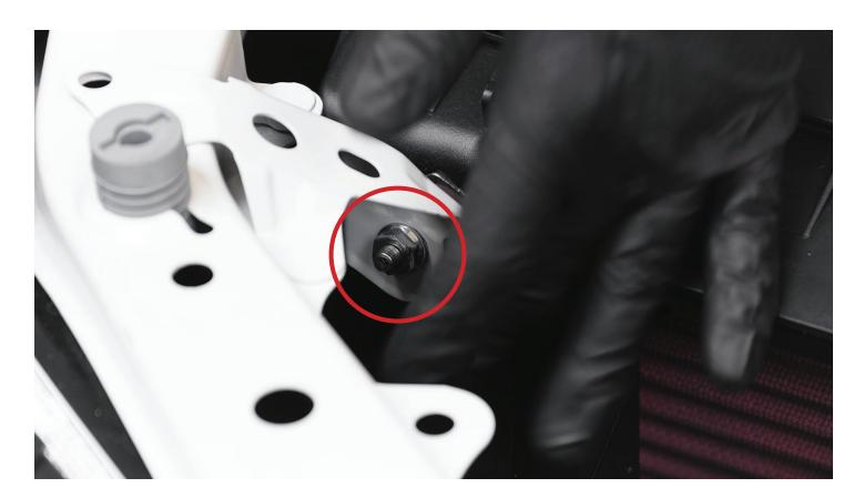
**STEP 25** - Reinstall the intake duct back onto the airbox and replace the two pop-fasteners into the radiator cover to secure the duct in place.
