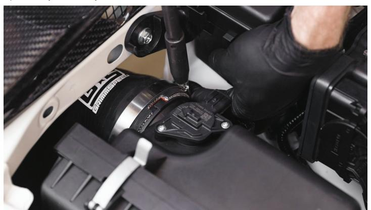
**STEP 23 -** Reconnect the witing harness to the MAF sensor and clip the plastic fastener back into place on the back of the airbox to prevent the wiring from moving around at all.
