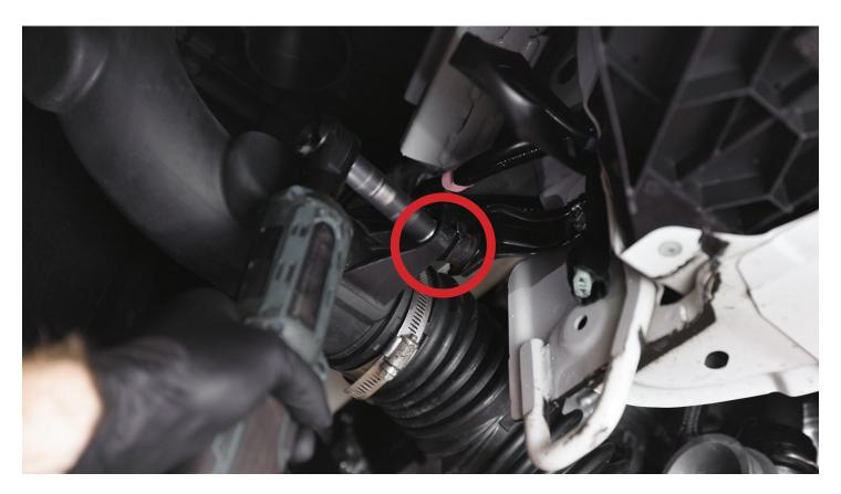
**STEP 6 -** Using a flathead screwdriver to remove the 2 plastic clips securing the factory airbox duct from the top of the engine bay. Once the clips are removed, the duct will lift out of the airbox.
