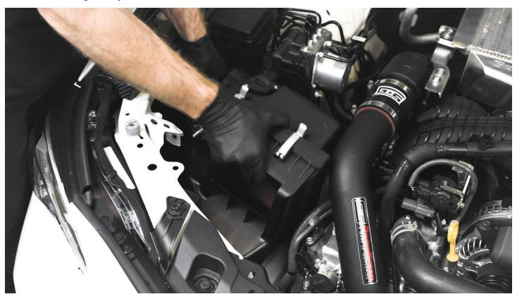
**STEP 11 -** With the airbox removed, you can pull the factory plastic post-MAF pipe out from under the frame rail.
