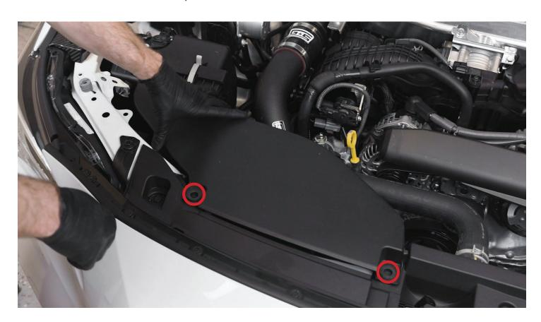
**STEP 26 -** With everything else in place, reinstall the steel skid plate and plastic under tray underneath the car using all of the fasteners your removed in steps 1 and 2. Once those are back in place, you are good to lower your car back down and hit the road!
