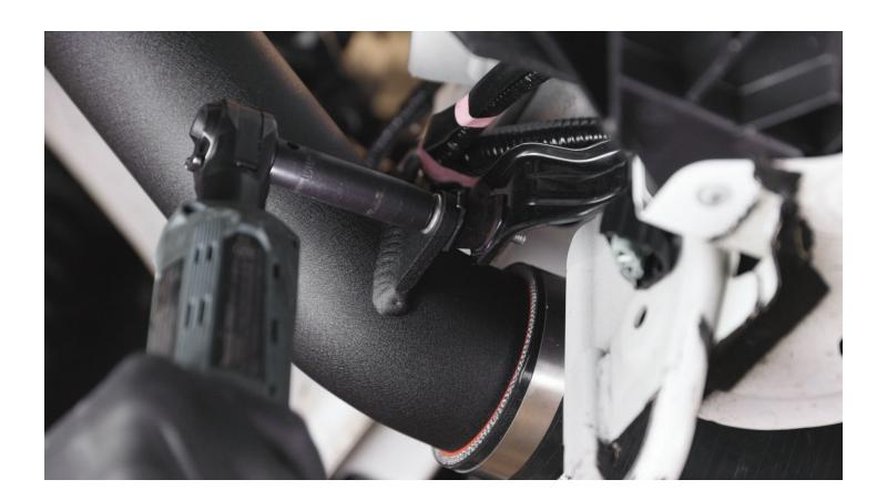
**STEP 19 -** Back in the engine bay, twist the upper coupler into place so that the air-box side of the coupler is paralell with the upper fender. Once this is aligned, tighten the hose clamp securing the elbow coupler to the Post-MAF Pipe.
