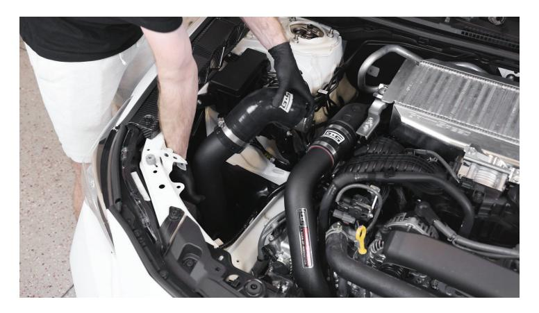
**STEP 15** - Back under the car, pop the lower coupler onto the turbo inlet aligning the bump on the inlet flange with the notch cut out of the coupler. Also, insert the stud from the rubber isolator into the hole in the mounting tab on the pipe.
