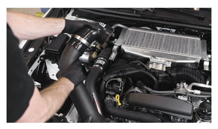
**STEP 14 -** Install the new pipe into the car by sliding the lower end in first from the top. Try to get the lower coupler as close to the turbo inlet as you can.
