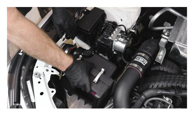
**STEP 21 -** Reinstall the two 12mm bolts we removed earlier to attache the airbox to the frame rail. Start these bolts by hand first before tightening with a wrench or power too to avoid crossthreading or stripping out the threads in the frame rail.
