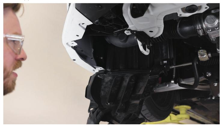
**STEP 4 -** Loosen up the hose clamp connecting the factory intake pipe to the aluminum turbo inlet.
