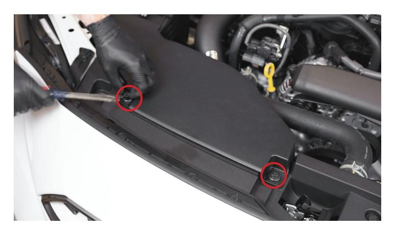
**STEP 7 -** With an extension, remove the 2 12mm bolts securing the lower airbox to the fram rail.
