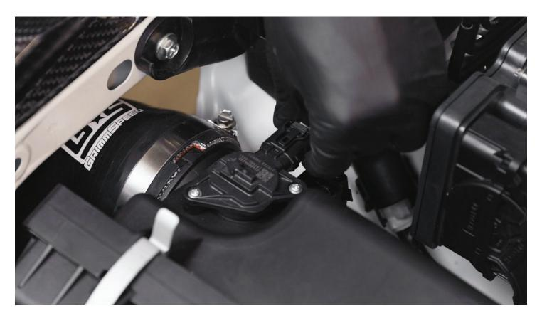
**STEP 24** - Reinstall the 10mm nut onto the stud on the airbox. Once again, snug this nut down by hand to avoid damaging the the threads and then tighten it the rest of the way with a 10mm wrench.
