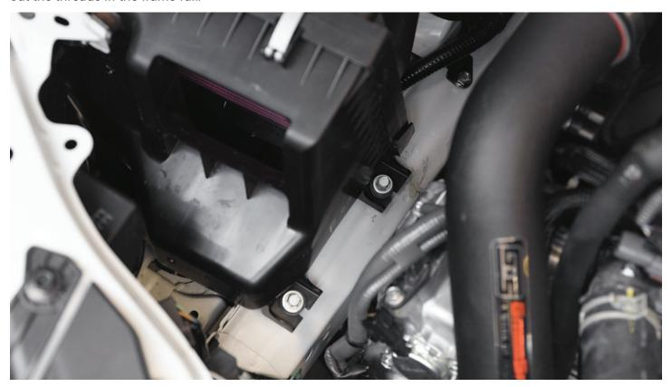
**STEP 22** - Ensure that the notch in theupper elbow coupler alignes with the molded dimple on the airbox. Once this is aligned and the coupler is fully seated, tighten down the final clamp to secure the Post-MAF Pipe assembly to the factory airbox.
