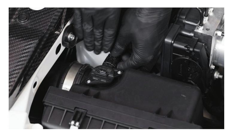
**STEP 9 -** Loosen up the upper worm clamp on the intake pipe.
