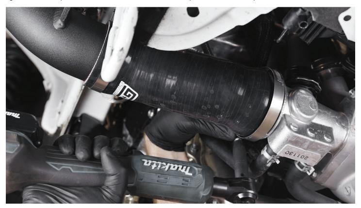
**STEP 18 -** fully tighten the 10mm nut to secure the Post-MAF Pipe into place under the car.
