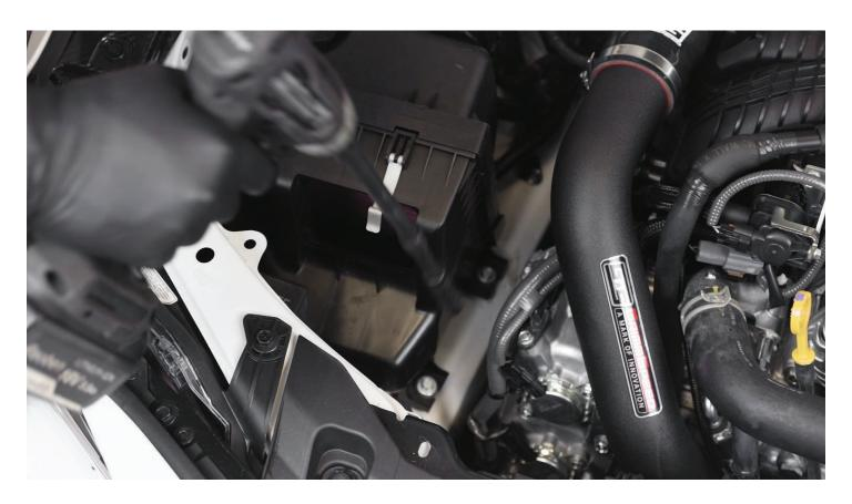
**STEP 8 -** Unplug the engine harness from the MAF sensor on the airbox. You will also want to unclip the wiring loom from the back of the airbox.
