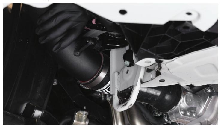
**STEP 16 -** Loosely thread the 10mm nut into place to hold the pipe in place before tightening down the lower pair of hose clamps.
