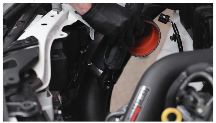
**STEP 20 -** You can drop drop the OEM airbox assembly back into the engine bay, taking care to align both the elbow coupler with the airbox outlet and the threaded mounting stud with the tab above the headlight.
