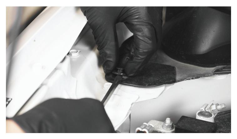
**STEP 2 -** Remove the painted 10mm bolt right in front of the clip that was just removed.
