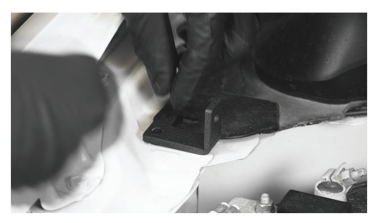
**STEP 4 -** Secure the bracket in place using one of the longer 10mm bolts that was incuded in your hood strut kit.
