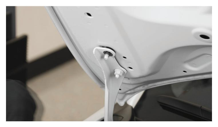
**STEP 8 -** Slot the hood bracket into place on the hood hinge as shown below, inserting the slotted end in between the hood hinge and the nut you loosened in the last step. With the bracket in place, you can reinstall the upper nut and retighten both hinge nuts.
