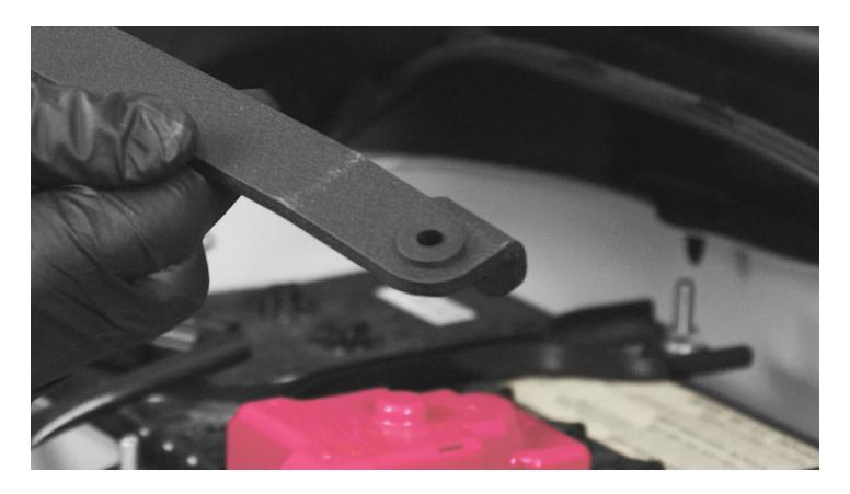
**STEP 7 -** On the hood hinge, completely remove the upper 12mm nut that secures the hinge to the hood. You don't need to completely remove the lower nut, but break it loose and back it off ~1/4".
