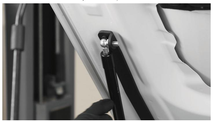
**STEP 10 -** Repeat the same step from above with the lower end of the strut on the fender side bracket. With the lower end in place, go back and fully tighten the upper and lower 1/2" strut nuts holding the ball stud with a thin 1/2-inch wrench.
