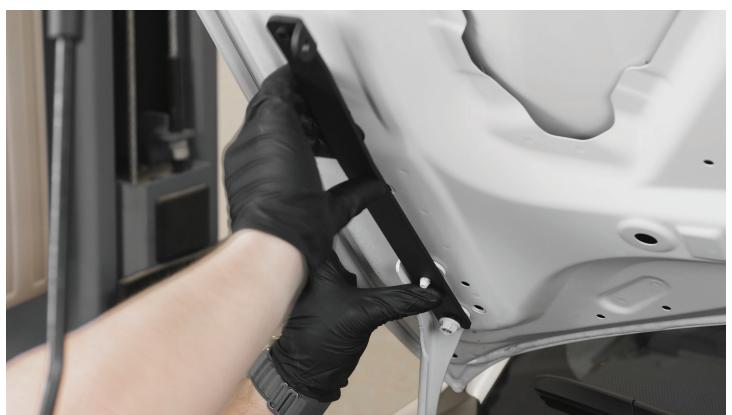
**STEP 9 -** With your hood bracket securely bolted in place, grab one of the hood struts and install it into the upper bracket as shown below with the threads of the ball joint pointing towards the center of the chassis. Use one of the included 1/2" nuts to loosely hold this end in place.
