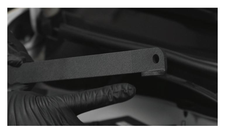
**STEP 6 -** Install one of the included rubber grommets into the bracket through the larger hole with the flat side of the grommet facing AWAY from the bent tab as shown below.
