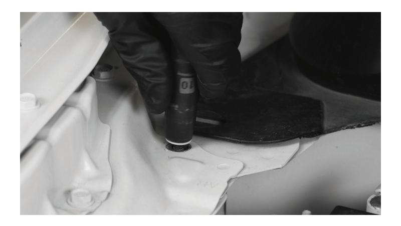
**STEP 3 -** Install the lower strut bracket as shown below. The narrow bent tab should be inserted into the hole left from the plastic trim clip.
