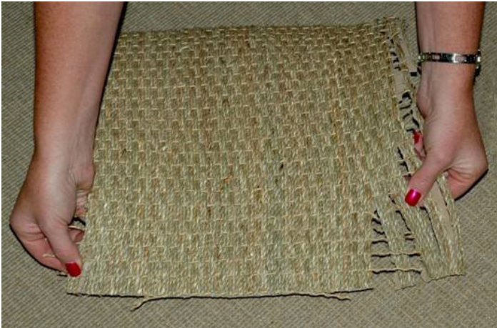
Standard Latex is light weight, with minimal dimensional stability and will pull apart.
