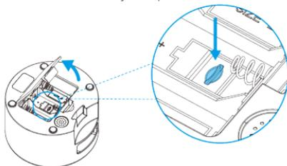
2) Insert the TF card in the direction shown. Slide it in until it clicks into place. Do not force or apply excess force when inserting the TF card.
