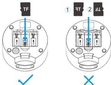
**Note: Insert the TF card correctly. Not doing so can cause a malfunction.**
