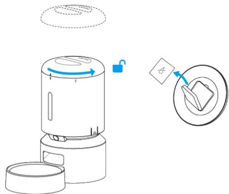
3. Pull the notches on both sides outward a little and then up to remove the food tank.
