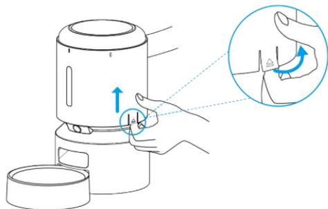
4. Twist anticlockwise to remove the tank base.
