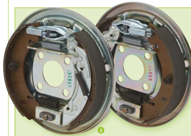
1 P000160 Brake assembly. 250 x 40 RH & LH - Bolt on type backplates pre-assembled with shoes, springs etc (From Jan 1996 - March 2014). Unequally spaced holes in a rectangular pattern.
