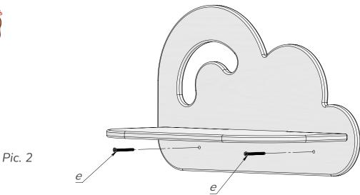
If you have a concrete wall - attach the assembled construction to the wall using self tapping screws (e) together with dowels (c), if you have a dry wall, use a dowel (d). See Pic.2.
