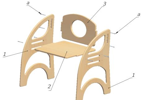
Take the seat (2) and the back (3) and using the confirmation screws (a) and a hex key (b) connect the sidewalls (1). See Pic. 1
