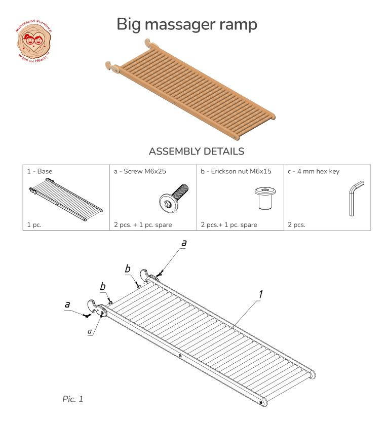
Take the base (1), turn the hooks 180 degrees. Next, with the help of screws (a), nuts (b) and two keys (c), screw it to the guide base and tighten the other screws (a) See Pic. 1.
