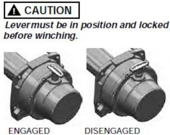
**DO NOT ATTEMPT to pull a load until the drum is properly engaged.**
