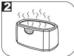
If unit has been working 3 cycles, it's better to stop over 10 minutes, in order to prolong the using life.
