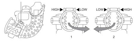
By simultaneously adjusting the left and right wheels in different directions, the machine can launch different curve balls:
