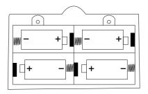
Assemble the battery according to the positive "+" and negative "-" signs.
