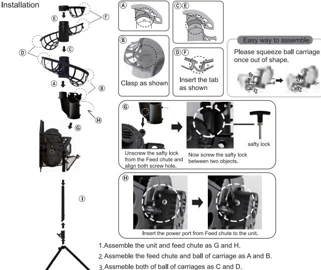
4 Assmeble the top of carriage and ball of carriage as E and F.
