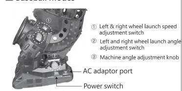
① Left & right Wheel launch speed adjustment switches Perform hook ball by adjusting speed as shown
