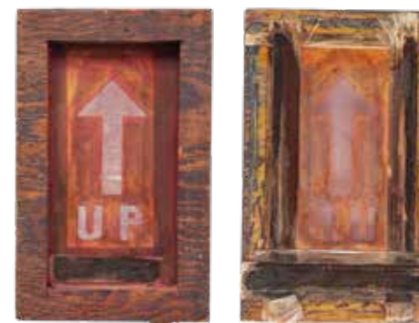
Screens used to print on wooden boxes at the factory of Paul-Émile Larocque
