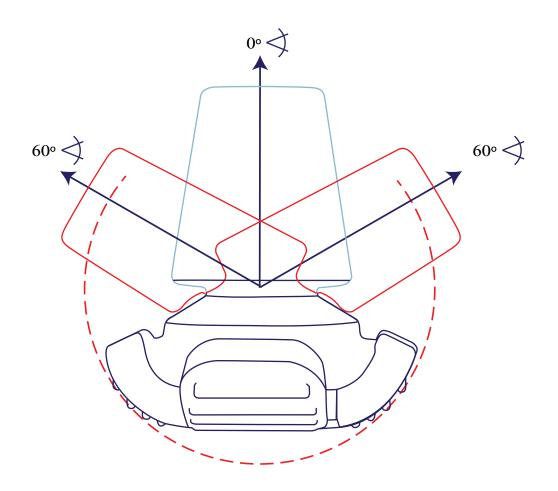
Articulated neck allows the upper body of the cane to emulate the tibial navicular joint, allowing a much more safe and comfortable gait.
