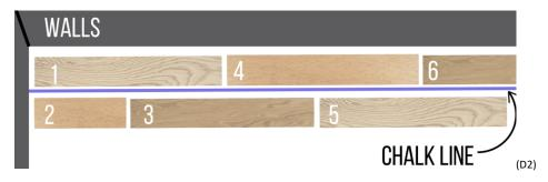
**Important:** For successful installation, use diagram #2 above and install the boards in the order as indicated for the first two rows and use D1 sequence example to determine proper measurements and make sure your installation is starting on the straightest possible line. You will install from left to right.
