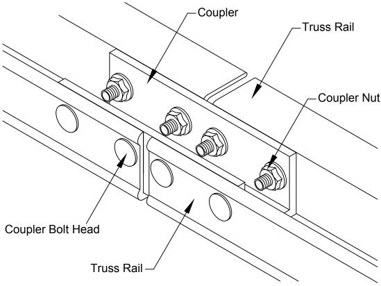
Install all 16 bolts and nuts (per truss connection) before wrench tightening (about 9 ft-lbs). Assemble all trusses referring to 2.1 General Arrangement and 3.1 Truss Configurations.
