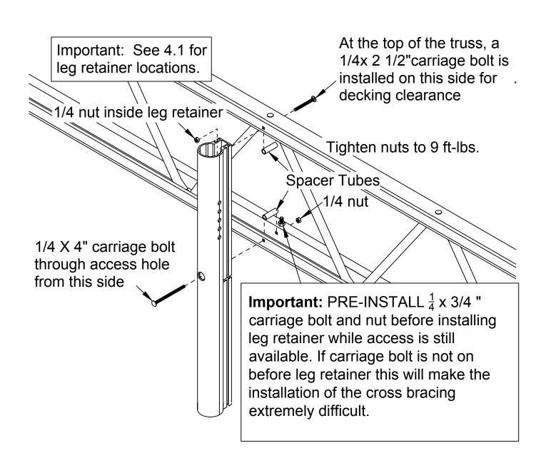
Note: Do not fully tighten bolts and nuts until all components (sections 4.2, 4.2.1, and 4.3) have been installed, unless specified otherwise.
