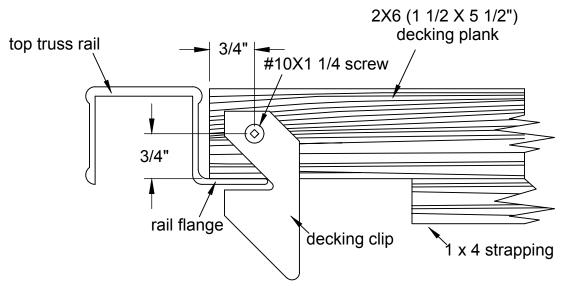
6.5 Top of Rail Decking Retaining Clip Installation
