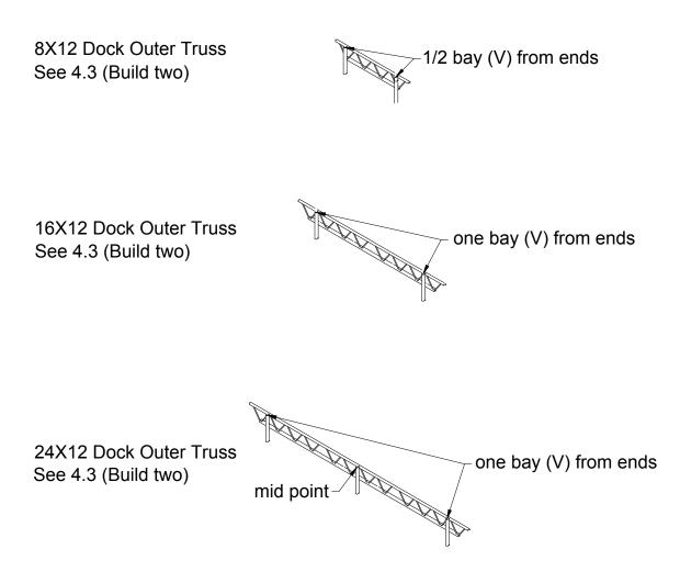
The two inner trusses for 12' wide docks (2 per 8X12, 16X12 and 24X12) and the 12' cross trusses (2 per 8X12 and 16X12, 3 per 24X12) do not receive leg retainers.
