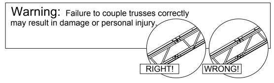
Selecting a flat work area may ease the assembly of the precision manufactured trusses and couplers. Using leveled saw horses and an assistant is an acceptable substitute.
