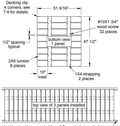
decking panels supported by rail flange between dock trusses
