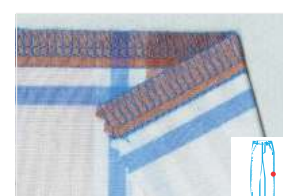
Six threads sewing P15
