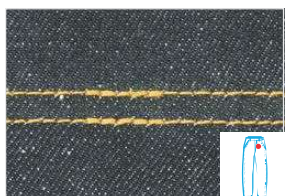
Double needle straight stitch P08
