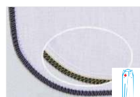
Five threads pocket double chain rolling stitch P15
