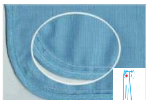
Pocket double chain rolling stitch P15
