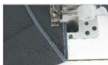
Edge cutter and tape binner (JK-5559G-T)
