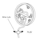
Step 5. Make sure the waterproof gasket is in a good position. Close the cover and tighten the screws.
