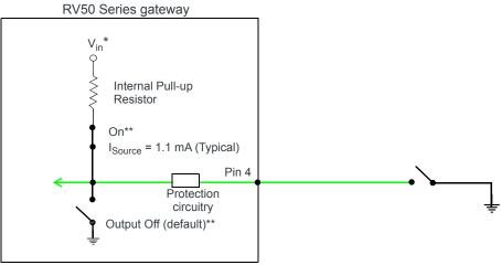
\*Depending on the load, this value can range from Vin to Vin - 2.5 V. \*\* Configurable on the ACEmanager I/O tab
