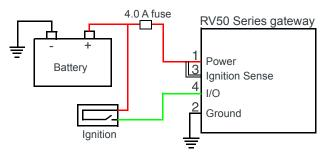
Figure 3-7: Alternate Vehicle Installation
