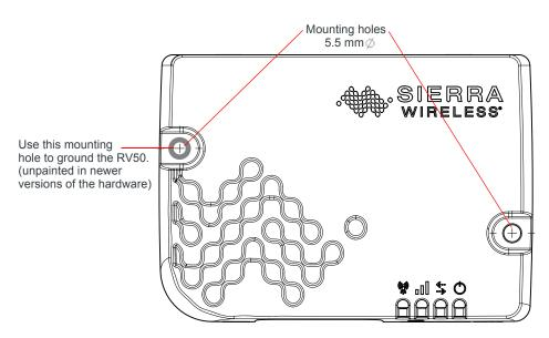
Figure 3-4: Mounting and Grounding the RV50
