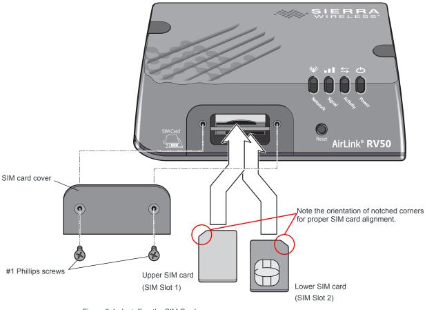
Figure 3-1: Installing the SIM Card
