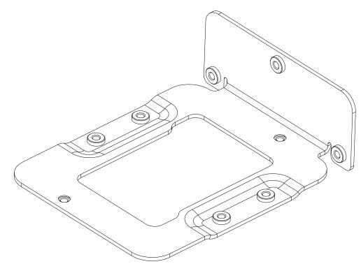
Figure 3-20: DIN Rail Mounting Bracket
