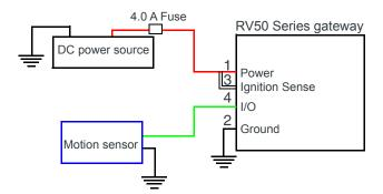
Figure 3-9: Fixed Installation with I/O
