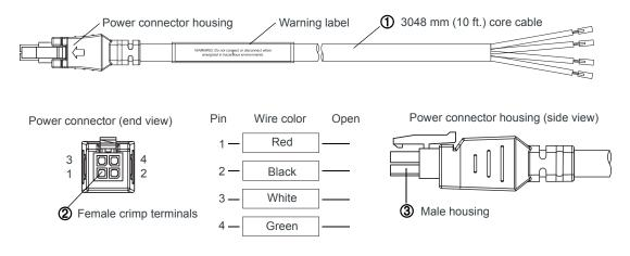
Figure A-1: DC Cable Specifications
