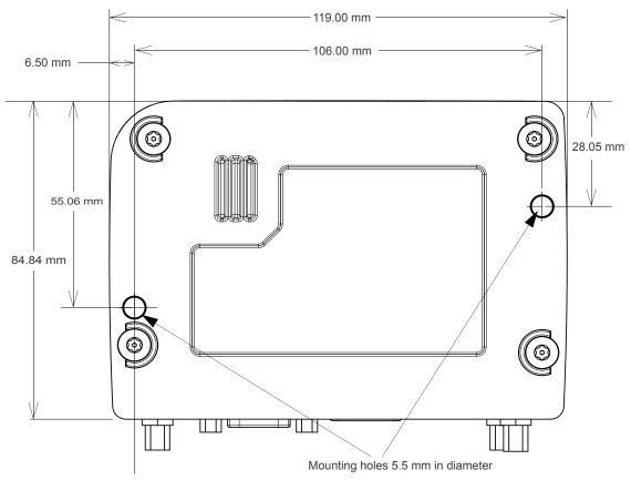
Figure 3-19: RV50 Series Gateway Mounting Bracket for Flat Surfaces
