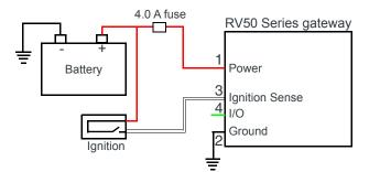
Figure 3-6: Recommended Vehicle Installation
