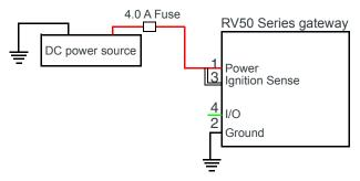
Figure 3-8: Fixed Installation without I/O
