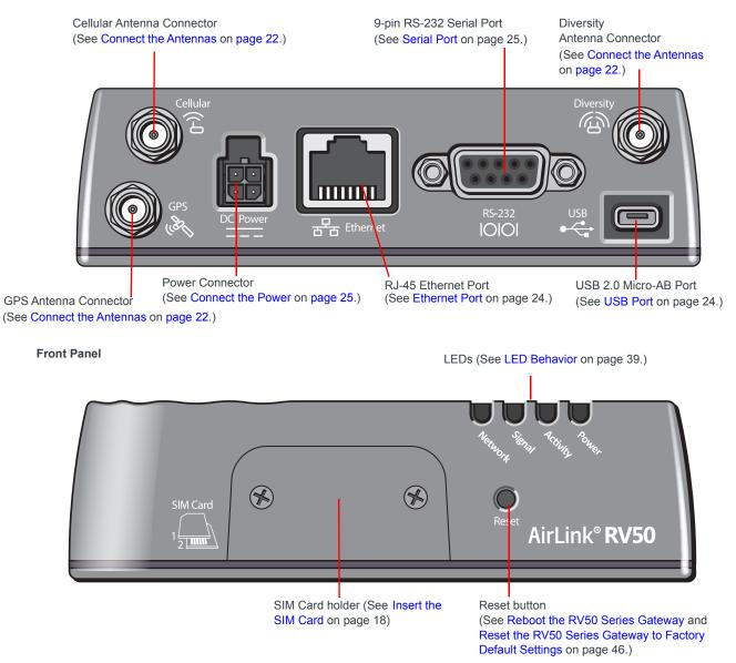
Figure 1-1: RV50 Series Gateway Connectors, LEDs and SIM Card Holder
