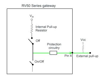
Figure 3-16: Digital Output/Open Drain
