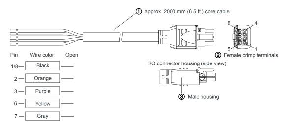
Figure A-2: I/O Cable Specifications
