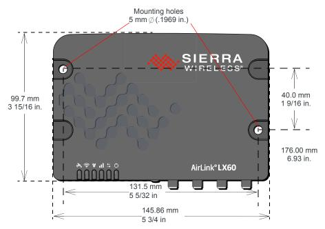
Figure 2-2: Mounting and Grounding the LX60
