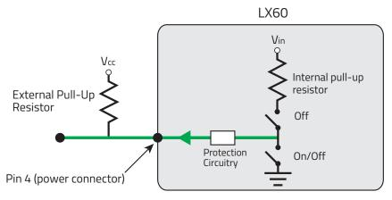
Figure 2-17: Digital Output/Open Drain
