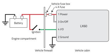
Figure 2-9: Alternate Vehicle Installation
