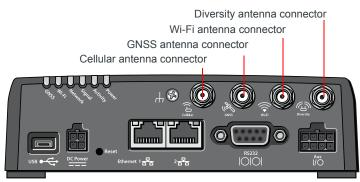
Figure 2-4: Antenna Connectors
