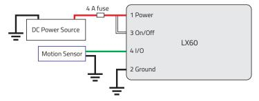
Figure 2-7: Fixed Installation with I/O
