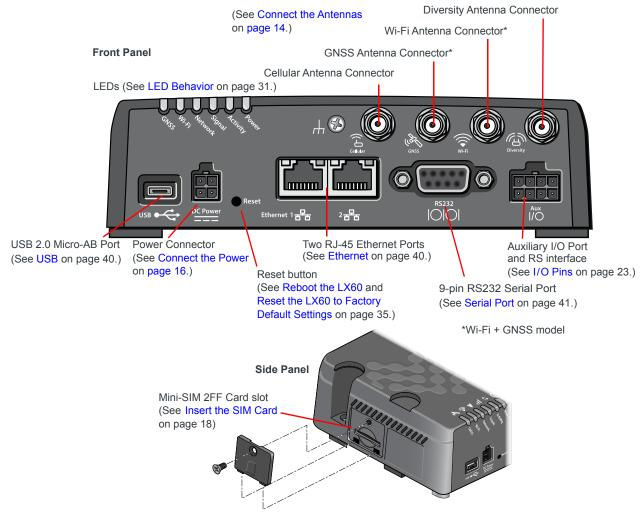
Figure 1-1: LX60 Connectors, LEDs and SIM Card Holder
