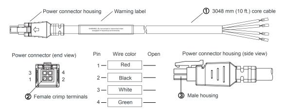
Figure A-1: DC Cable Specifications
