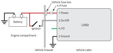
Figure 2-8: Vehicle Installation Option 1
