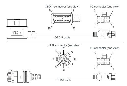
Figure A-3: Vehicle Bus Cables
