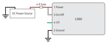
Figure 2-6: Fixed Installation without I/O
