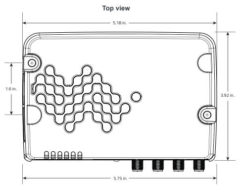
Figure 3-3: LX60 Mechanical Specifications
