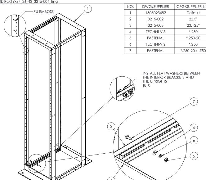
CFG/SUPPLIER NO. **DESCRIPTION** QTY FRAME (19 x 84) 2 **EXTERIOR BRACKET** 4 INTERIOR BRACKET 4 32 FLAT WASHER 1/4" 24 HEX NUT 1/4-20 SPLIT LOCK WASHER 1/4" 24 \*.250-20 x .750 8 HEX BOLT 1/4-20 x 3/4
