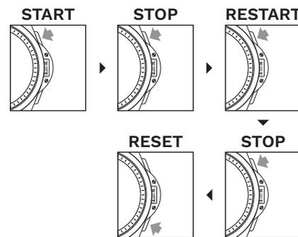
Restart and stop of the stopwatch can be repeated by pressing the button A.
