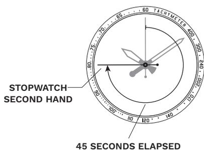
**Note:** The tachymeter indications may appear on dial ring, rather than on the outer bezel (depending on model).
