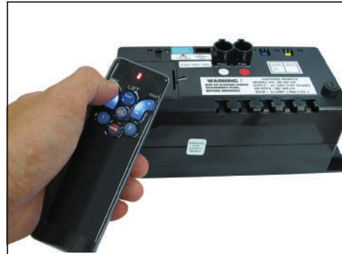
Figure 2: A flashing Green LED indicates the control box has received the remote control signal.
